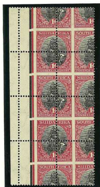
Freak caused by faulty alignment of perforating comb.
